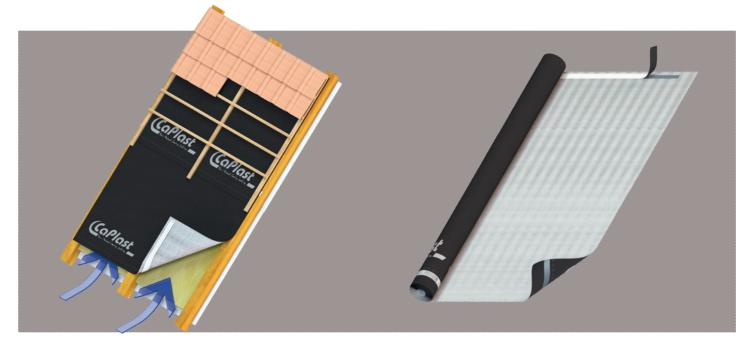
CaTop M 120 SK is a diffusion permeable, standard-compliant sarking membrane, in accordance with DIN EN 13859-1, that has two double-sided self-adhesive strips, applied both sides. Also available without self-adhesive strips, as CaTop M 120. The multi-layer membrane is made of polypropylene non-woven fabrics separating an inner-lying functional membrane.
