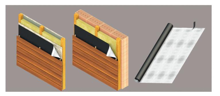
CaWrap UV 200 SK consists of a PES non-woven material and an innovative, diffusion permeable polyurethane coating, which provides long-lasting UV protection. Driving rain or snow are effectively kept out by the insulating layer. The smooth surface of the façade membrane allows incident or infiltrating moisture to safely and securely run off. This membrane is also available without self adhesive strips.
