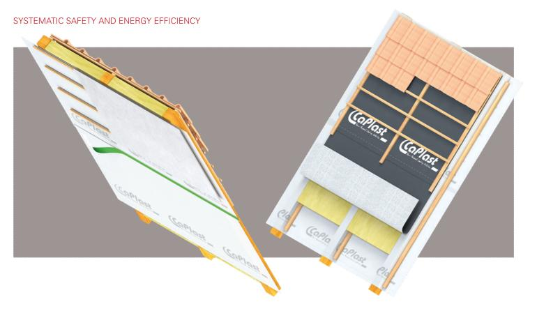
CaVap 2 is an all-round vapour barrier for all roof and wall constructions. The vapour barrier consists of a polypropylene non-woven fibre with a copolymer coating. Available with and without self-adhesive strips (SK). CaVap 2 is translucent and thus allows the rafters behind the vapour barrier to remain visible. Thanks to its high flexibility, CaVap 2 can also easily adjust to complex details.
